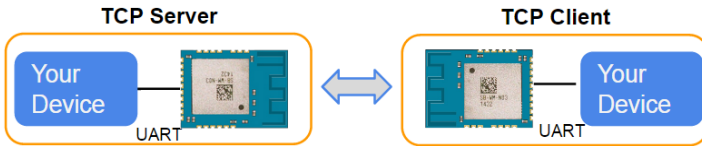
Example: direct link for cable replacement
