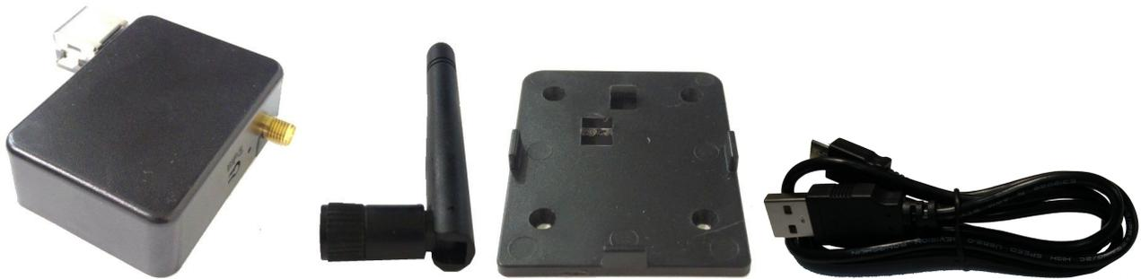
There are one iGS02E unit, one 1M USB cable, one holder, and one 2dBi dipole antenna included in one full shipping package. iGS02E is powered by a standard micro-USB cable, rated at 5V&500mA. You can power this device with a standard smartphone charger or the USB port of any host device that can support 500mA or above.
