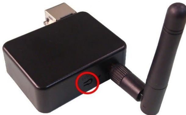
It is used to reset to default settings. In case you need to go back to the original settings, keep pressing the reset/default button in your device for over 5 secs no matter in which mode the device is. The Ethernet LED will be turned off and when you release the button, the iGS02E will reboot to its default settings.
