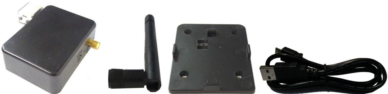
There is one iGS02E unit, one 1M USB cable, one holder, and one 2dBi dipole antenna included in one full shipping package. iGS02E is powered by a standard micro-USB cable, rated at 5V&500mA. You can power this device with a standard smartphone charger or the USB port of any host device that can support 500mA or above.
