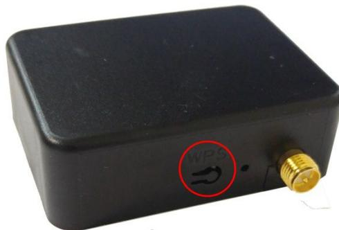
It is used to act WPS, reset to default settings, and OTA (over-the-air FW upgrade). Below is how it functions.
