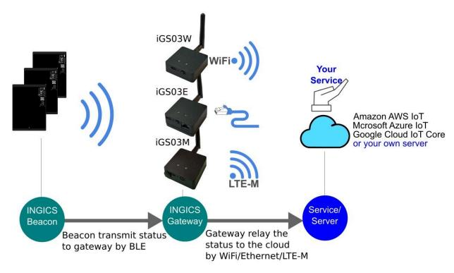
Note: iGS03W/E/M are the 3rd generation of beacon gateway in WiFi/Ethernet/LTE-M interface.
