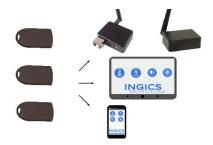
2. By using iGS01S or iGS02E beacon gateway to receive the beacon message and send to the cloud server, user is able to access and manage the data anytime, anywhere.
