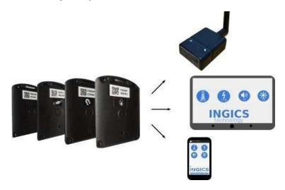
2. Use iGS01 beacon gateway to receive the beacon message and send it to the cloud server. You can then access and manage the data anytime anywhere.
