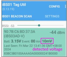
The detected voltage range is 0~24000mV.
