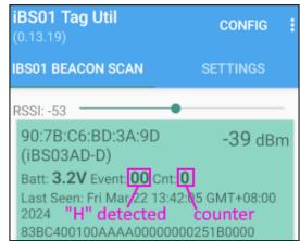
Event 00: "H" detected or no connection Event 40: "L" detected Counter: For each "L" detected, it will add 1 in the counter
